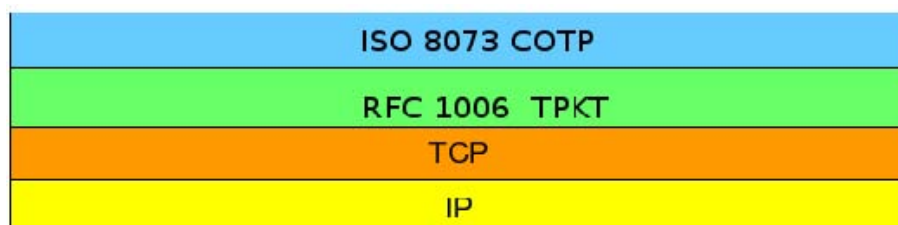
Figure 4: The MMS communication stack as Wireshark detects it
